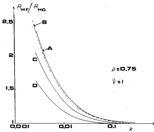
Figure 3 Variations in the Hall coefficient ratio  $R_{HF}/R_{HO}$  with the reduced thickness  $k$  (for  $p = 0.75$  and  $\nu = 1$ ) under the influence of the magnetic field,  $H$ . For curves A, B, C and D,  $\alpha = 0.01, 1, 4$  and  $10$  respectively.
