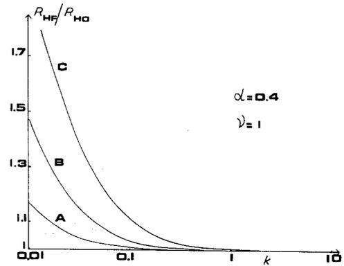
Figure 5 Variations in the Hall coefficient ratio  $R_{HF}/R_{HO}$  with the reduced thickness,  $k$  (for  $\alpha = 0.4$  and  $\nu = 1$ ) under the influence of the specularity parameter,  $p$ . For curves A, B and C,  $p = 0.9, 0.75$  and  $0.5$  respectively.
