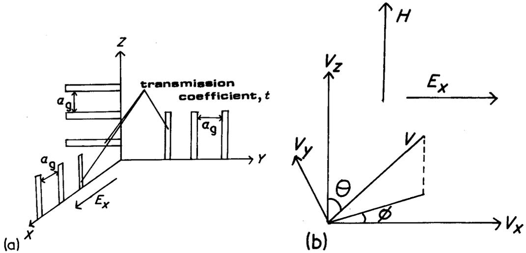
Figure 1 Geometry of the model; (a) the grain model and (b) the velocity co-ordinates.
