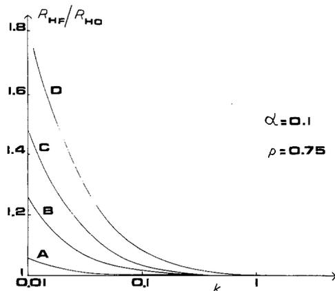
Figure 4 Variations in the Hall coefficient ratio  $R_{HF}/R_{HO}$  with the reduced thickness,  $k$  (for  $p = 0.75$  and  $\alpha = 0.1$ ) under the influence of the grain parameter,  $\nu$ . For curves A, B, C and D,  $\nu = 0.1, 0.4, 1$  and  $4$  respectively.
