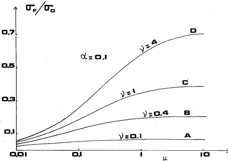
Figure 2 Variations in the conductivity ratio  $\sigma_F/\sigma_0$  with  $\mu$  (for  $\alpha = 0.1$ ) under the influence of the grain parameter,  $\nu$ . For curves A, B, C and D,  $\nu = 0.1, 0.4, 1$  and  $4$  respectively.
